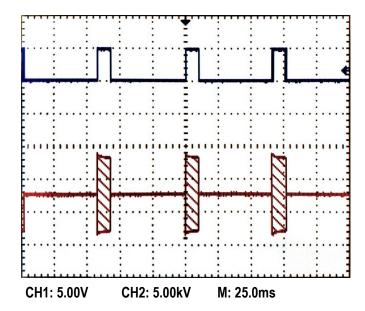
**Channel 1:** 10 ms "train" pulses applied to Input D, rear panel interface connector.
